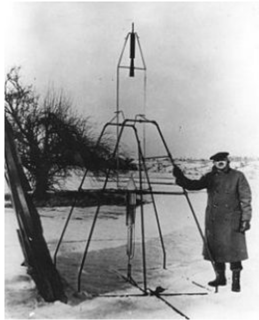
Robert Goddard and his liquid fueled rocket. Pictured are Goddard, the rocket, and a launching frame (large triangular structure at bottom). March 16, 1926. Photograph courtesy WikiCommons.
