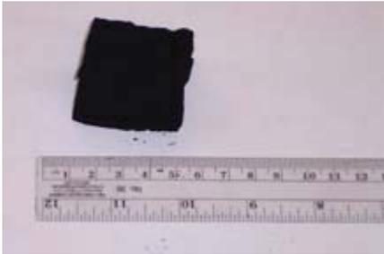
Figure 7.—Carbon aerosol gel.
