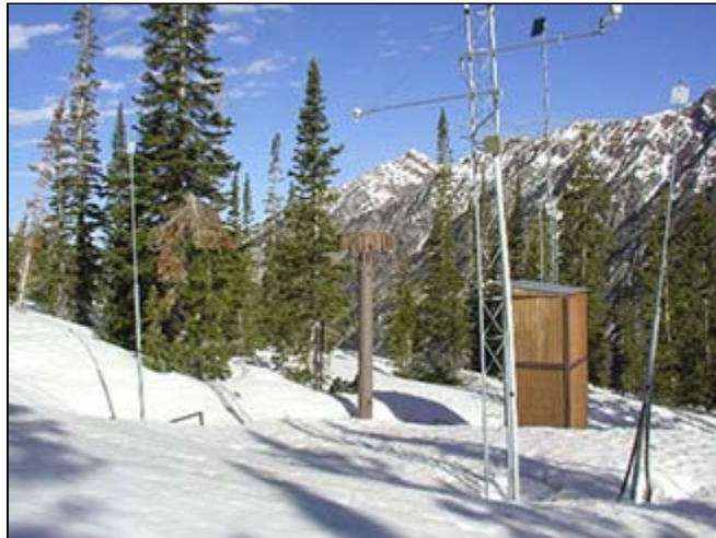
A series of monitors measures both snowpack and melt rates at a high-elevation site. Courtesy of the Natural Resources Conservation Service.
