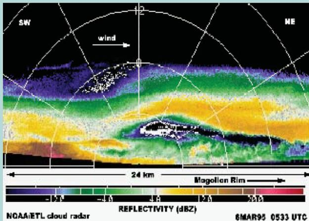
**Figure 2.** Observations from scanning cloud radar are converted to this “picture” of supercooled liquid in a wave cloud induced by the surrounding mountainous terrain. This is useful for locating good clouds to seed and then to monitor the ensuing changes in the cloud to better understand physical processes. **Source:** Reinking et al. (2000).
