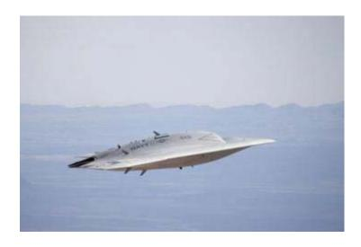
The X-47B Unmanned Combat Air System flew with its landing gear up for the first time on Sept. 7 during a test flight at Edwards AFB, Calif.
