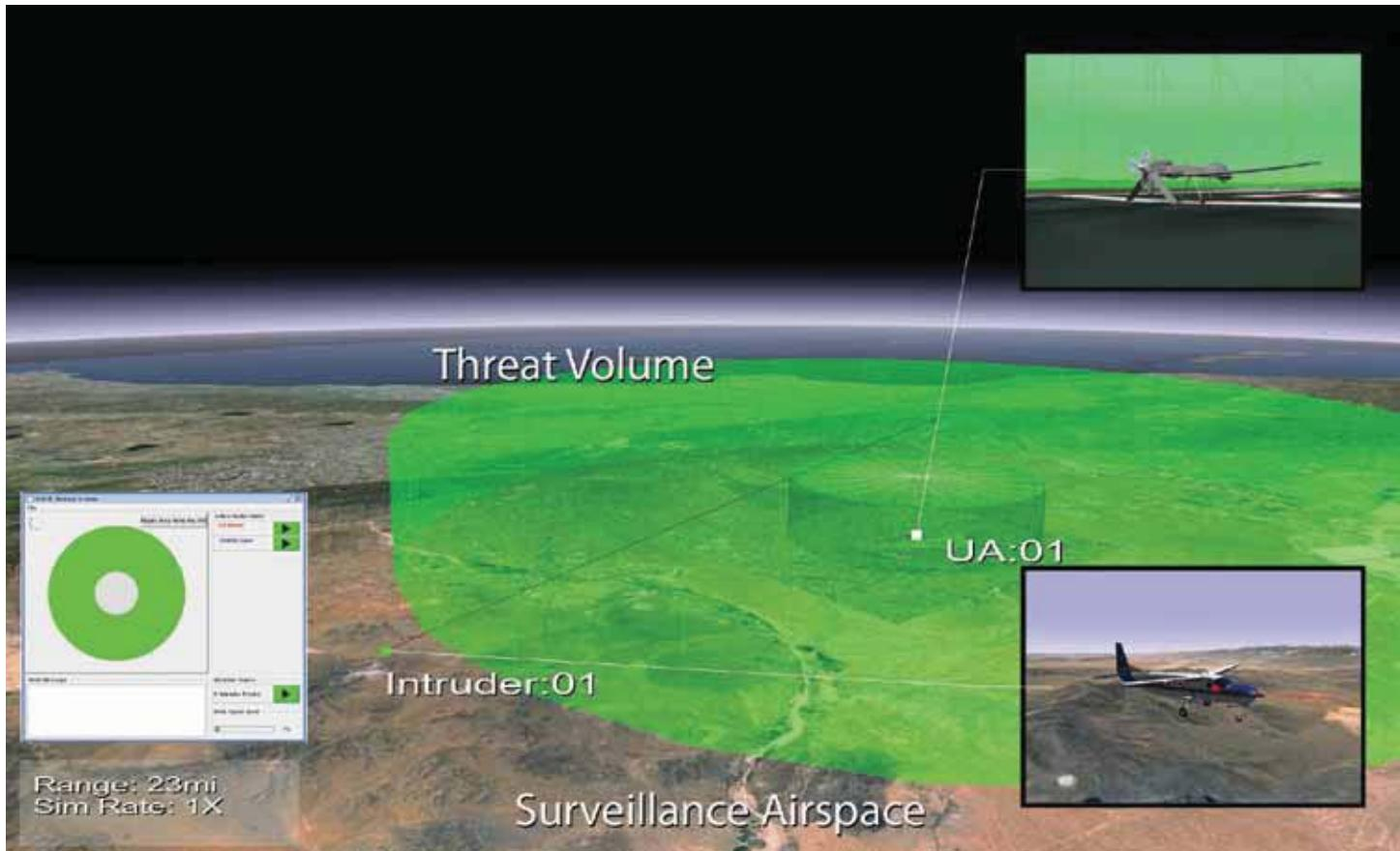
This image depicts an unmanned vehicle within its operational area, with an intruder approaching the threat volume. The status, shown by the Green Circle on the screen, means "authorized to fly."
