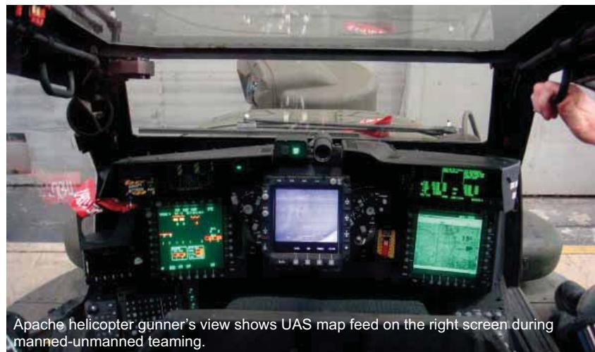
Apache helicopter gunner's view shows UAS map feed on the right screen during manned-unmanned teaming.
