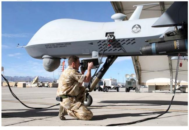
An avionics specialist checks out an MQ-9 Reaper before it prepares to fly from Creech Air Force Base, 2008. Photo: U.S. Air Force
