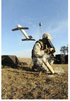
The Switchblade drone is designed to fit into a soldier's rucksack. It weighs less than 6 pounds and can take out a sniper on a rooftc without blasting the building to bits. The drone also enables so in the field to identify and destroy targets much more quickly by eliminating the need to call in a strike from large drones that may be hundreds of miles away. (AeroVironment / January 20, 2009)
