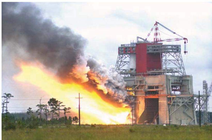
**Stennis operators conduct the first test-firing of a Saturn V booster stage – a cluster of five F-1 rocket engines – on Aug. 25, 1967.**
