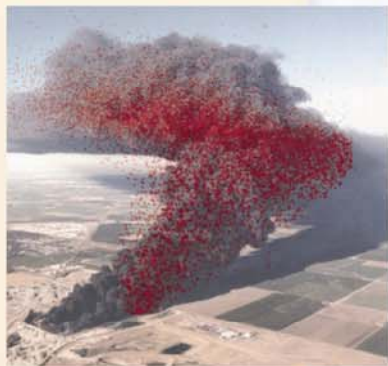
Smoke plume photograph with NARAC-simulated smoke particles in red. (Photo courtesy of Tracy Press.)
