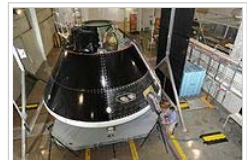
The Orion spacecraft is intended to be used for beyond low Earth orbit missions, shown here is the ground test article
