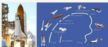
Discovery liftoff, 2008 Mission profile. Left: launch, top: orbit (cargo bay open), right: reentry and landing
