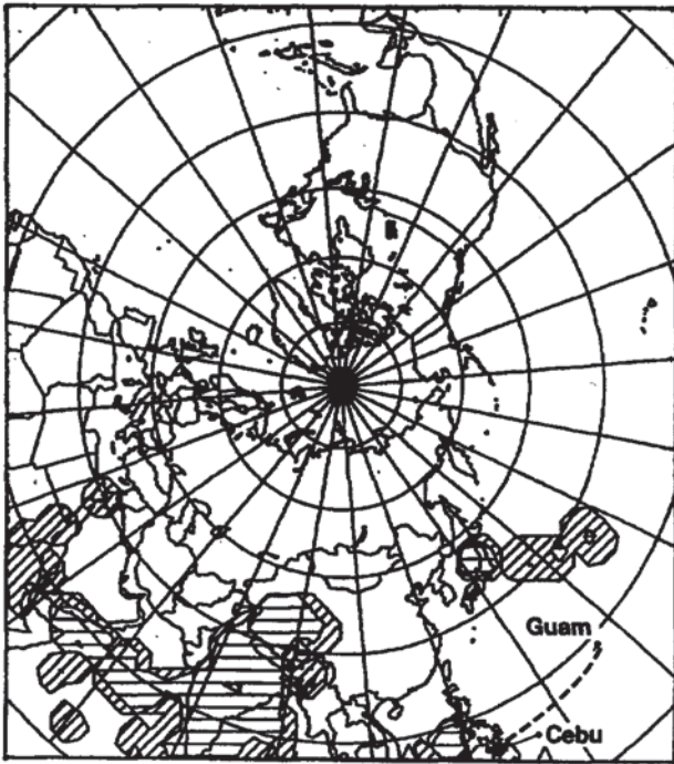
FIG. 10. One of the first Mt. Pinatubo ash-cloud advisory maps prepared for the U.S. Air Force on a hemispheric scale. This plot was for the 6- to 9-km layer at 0000 GMT on 20 June 1991.
