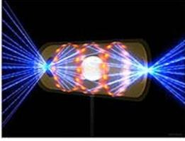
A rendering of a pellet hit by lasers to create nuclear fusion.
