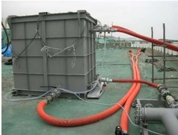
Fukushima Daiichi intake canal decontamination tank
