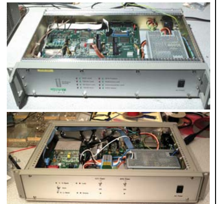
Fig 3: One of the new Programmable Receivers (top) and an associated IF Multiplexer (bottom).
