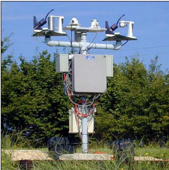
The U.S. Department of Agriculture maintains an extensive network of radiometers to monitor ultraviolet B (UV-B) radiation across the country. The one pictured above is in Beltsville, Maryland. (Photograph by Jeannie Allen)
