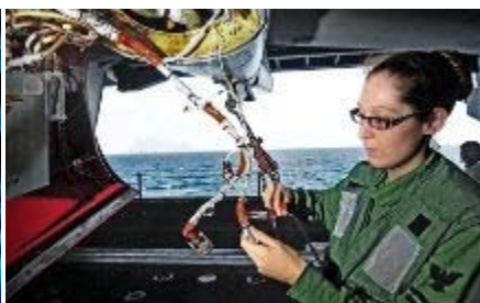
Aviation Electronics Technician spot ties wiring on an EA-6B Prowler
