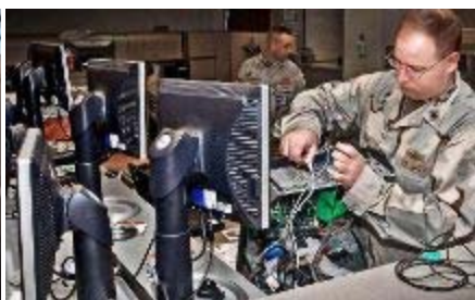
An Electronics Technician replaces a hard drive in a computer.
