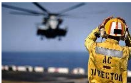
An aircraft director guides an MH-53E Sea Dragon to a landing spot aboard an amphibious assault ship.
