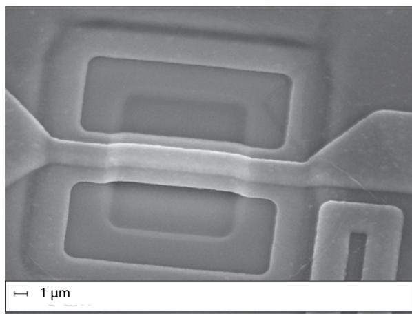
**FIGURE 15** SEM image of an arch bridge resonator. The laminated structure is comprised of a poly1 beam covered by a slightly wider poly2 stripe with a thin layer of interpoly oxide providing mechanical bonding between two poly layers, as well as electrical isolation.
