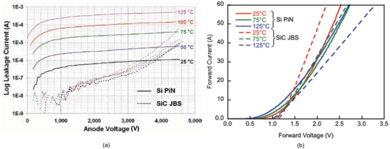
**FIGURE 8** (a) Comparison of the reverse blocking characteristics of Si PiN (solid lines) and SiC Schottky (dashed line) rectifiers as a function of temperature. (b) Comparison of the forward conduction characteristics of Si PiN (solid lines) and SiC Schottky (dashed lines) diodes as a function of temperature.
