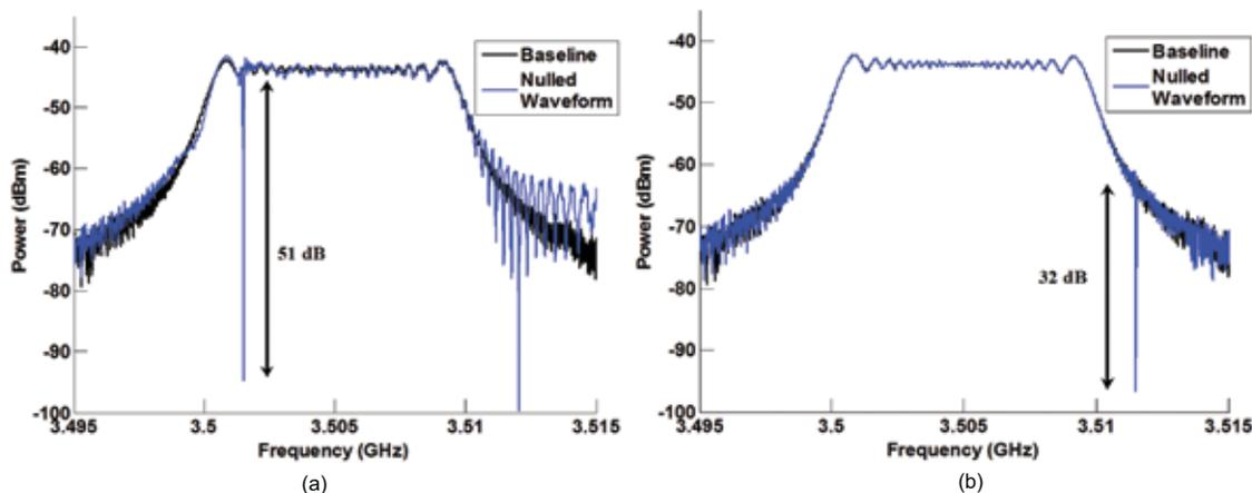
**FIGURE 5** (a) The in-band spectral null at 3.5015 GHz generated using the phase-coded linear frequency modulation (PC-LFM) approach. (b) PC-LFM result for an out-of-band null at 3.5115 GHz.
