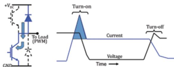
**FIGURE 7** Schematic drawing of a half-bridge circuit (left) and current-voltage waveforms as seen across the lower (blue) switch (right). During turn-on, the upper diode discharges into the lower switch, producing a large current transient (as illustrated by large arrow).
