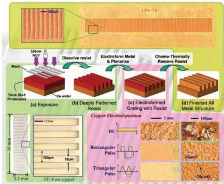
**FIGURE 11** The UV-LIGA process. (a) SU-8 is deposited on a polished copper wafer and exposed with UV, (b) the unexposed SU-8 is removed, and (c) copper is electroformed up between the crosslinked SU-8 patterns. Pulsed copper electroforming produces grain sizes far smaller than DC. (d) Finally, the SU-8 is removed.
