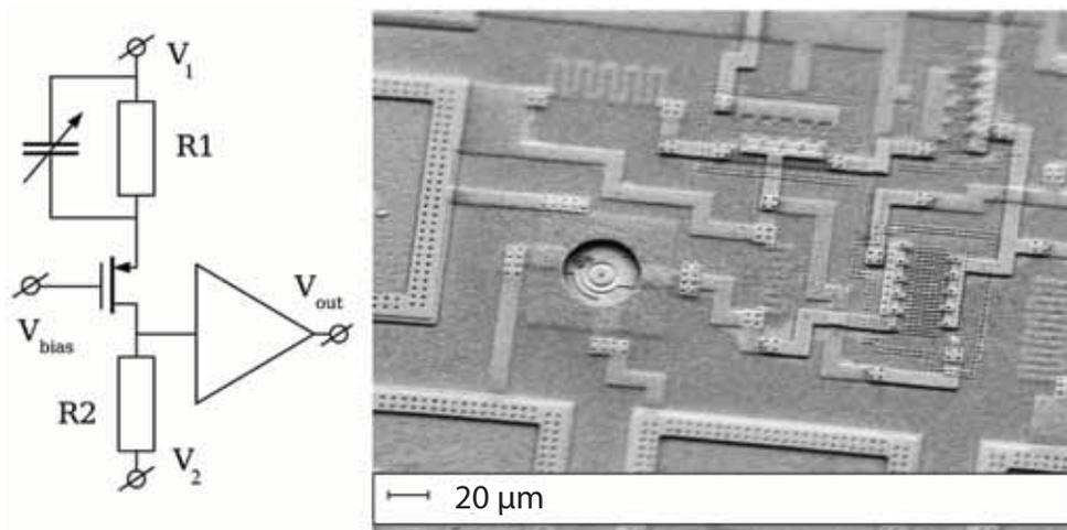
**FIGURE 14** Dome resonator integrated with a common-gate CMOS transimpedance amplifier. The dome resonator is depicted as a variable capacitor on the schematic diagram of the transimpedance amplifier (left).
