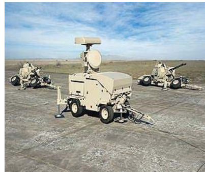
One weapon system -- two 5-kilowatt laser weapon modules -- was integrated into an air defense system using an Oerlikon Skyguard 3 fire control unit and a Skyshield gun turret.
