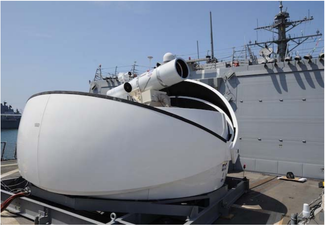
The Laser Weapon System (LaWS), shown here on the guided-missile destroyer USS Dewey. Photo: U.S. Navy
