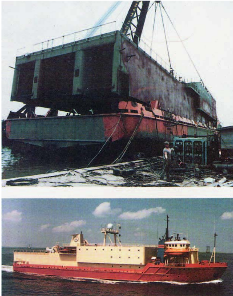
Figure 12. The R/V Cory Chouest . Under contract to APL, Edison Chouest Offshore of Louisiana purchased the M/V Tender Clipper , a Norwegian North Sea pipe carrier. In just four months, APL and Chouest transformed this platform into the most advanced ASW research and development platform in the world. The aft deck was outfitted with engineering, instrumentation, and berthing spaces by the addition of the "APL module" (top). The finished vessel was then reflagged and renamed the R/V Cory Chouest (bottom).
