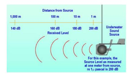
Received levels of sound underwater at 10, 100, and 1000 meters from a 200 dB source level referenced to one microPascal at one meter.
