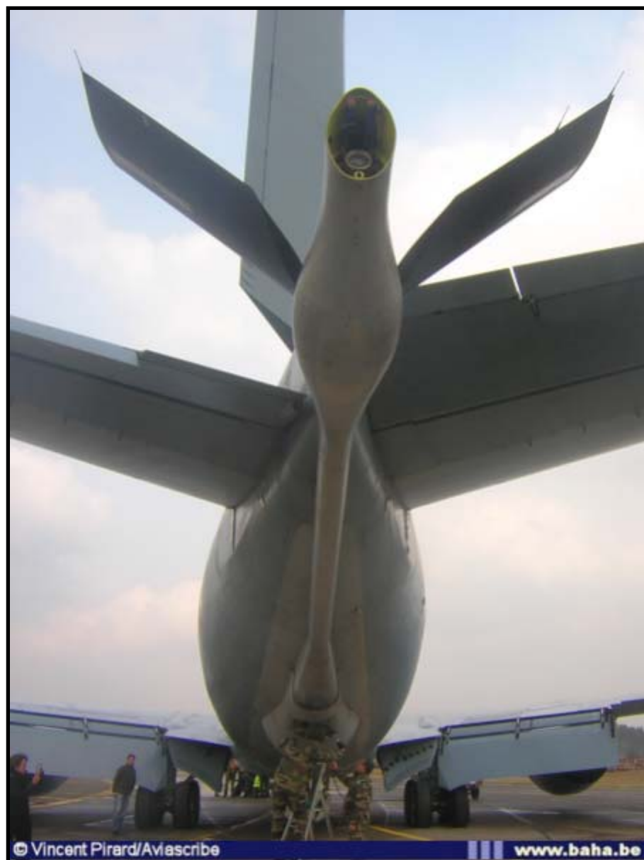
The rigid boom of C-135FR "93-CC"- s/n 63-8472. Ground crew members are cleaning the boomer's position windows before a mission.
