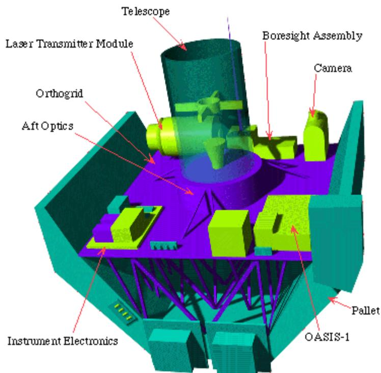
*Laser light, directed toward Earth, will bounce off of thin clouds, dust particles and the surface. Earth LITE's telescope receiver will "catch" that reflected light.)*
