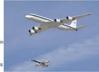
The NASA DC-8-72 is a four-engine jet transport aircraft that has been highly modified to support the agency's Airborne Science mission. The aircraft, acquired in 1985, is 157 feet long with a 148-foot wingspan. With a range of 5,400 nautical miles, it can fly at altitudes from 1,000 to 42,000 feet for up to 12 hours, although most science missions average six to 10 hours. The DC-8 can carry 30,000 pounds of scientific instruments and equipment.
