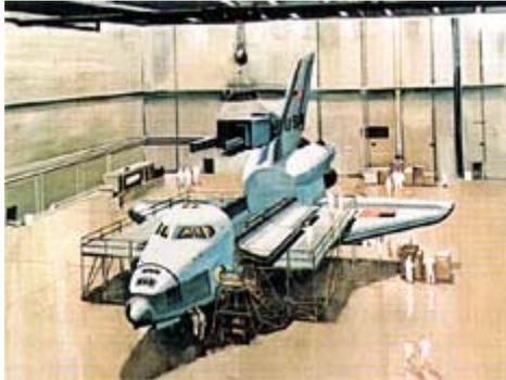
In a special change-out room, payloads are removed and different ones installed with the least delay.
