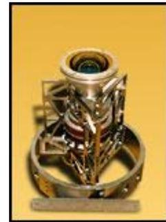
This calibrated lightning sensor uses a wide field-of-view expanded optics lens with a narrow-band filter in conjunction with a high speed charge-coupled device detection array. A Real Time Event Processor (RTEP), inside the electronics unit, is used to determine when a lightning flash occurs, even in the presence of bright sunlit clouds.
