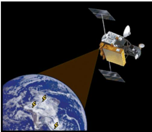
Weak lightning signals that occur during the day are hard to detect because of background illumination. The RTEP will remove the background signal, thus enabling the system to detect weak lightning and achieve a 90% detection efficiency.
