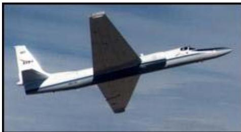
In order to determine the requirements for making optical measurements from space, U-2 and ER-2 high altitude airplanes have been used to study the electrical and optical characteristics of lightning activity in thunderstorms. Flying at an altitude of 20 km and at speeds of 200 meters per second, they are capable of flying over very large thunderstorms.
