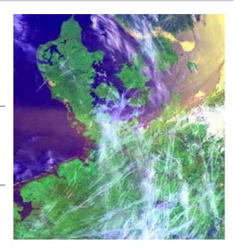
enough to be seen in visible satellite imagery. Sometimes a ship track appears as a band of enhanced cloud thickness embedded in stratus. Ship tracks are due to cloud condensation nuclei (CCN) in the ship's exhaust.
